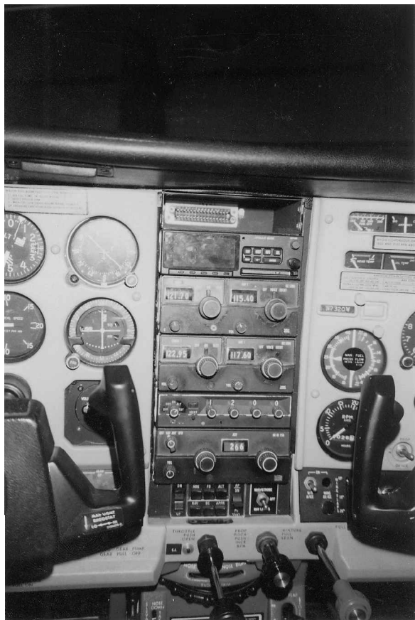
Fig. 1 Cessna-210 cockpit circa 1975 with dedicated gauges, 1990s loran and GPS installed in the avionics stack between the pilots (photograph by author).
