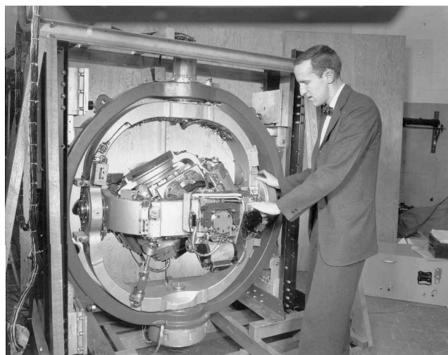
Fig. 5 Spire inertial navigator, circa 1956, five-gimbals; first aircraft inertial navigator (courtesy of The Charles Stark Draper Laboratory).
