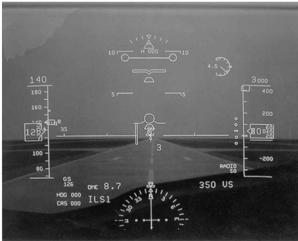
Fig. 14 HUD configured for takeoff, shows heading, airspeed, altitude, pitch, and other data (courtesy of Rockwell Collins Flight Dynamics).
