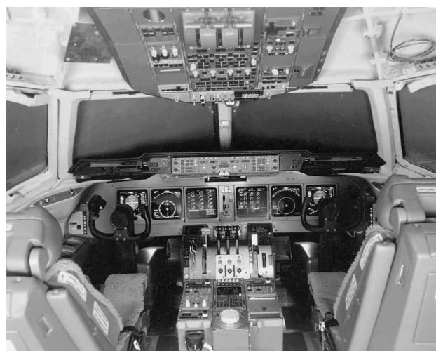
Fig. 13 MD-11 cockpit with multifunction displays and controls [courtesy of McDonnell Douglas Company (now The Boeing Company)].
