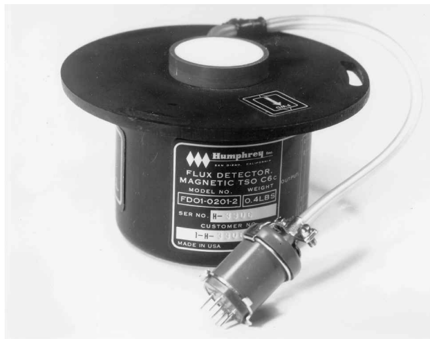
Fig. 3 Magnetic flux-gate sensor (courtesy of Humphreys).
