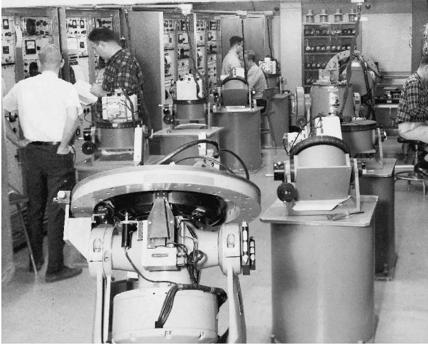
Fig. 8 Inertial instruments under test, 1950s: some tables are tilted to place their axis of rotation parallel to the Earth's spin axis; laboratory location is unknown to author.
