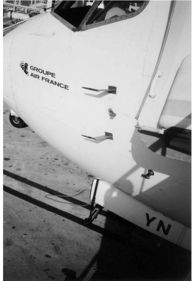
Fig. 4 Air-data sensors on Boeing 737: two pitots, one angle-of-attack, one temperature probe (photograph by author).
