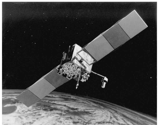
Fig. 9 GPS block IIF spacecraft (courtesy of The Boeing Company).
